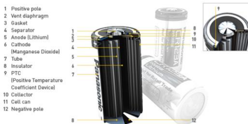
Figure 6: Cross-section of a cylindrical cell [13].
