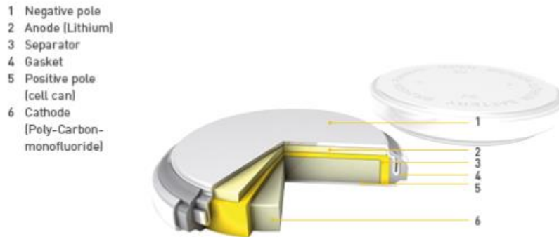
Figure 7: Cross-section of a button cell [13].
